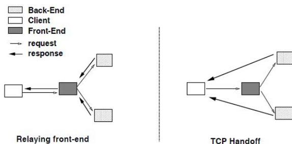
**Figure-3: Mechanisms for request distribution**
